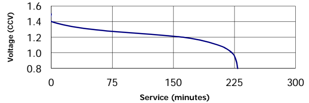
DIGITAL STILL CAMERA (DSC) .9/.4K mW 2/28 sec 10x per hour
